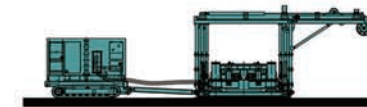
步骤二：连接反力叉和动力站 Step 2: Counterforce fork is coupled to the power station
